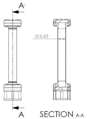
Custom Made; 6.63 inch ID, weld neck flange with 3/4 inch exit port
