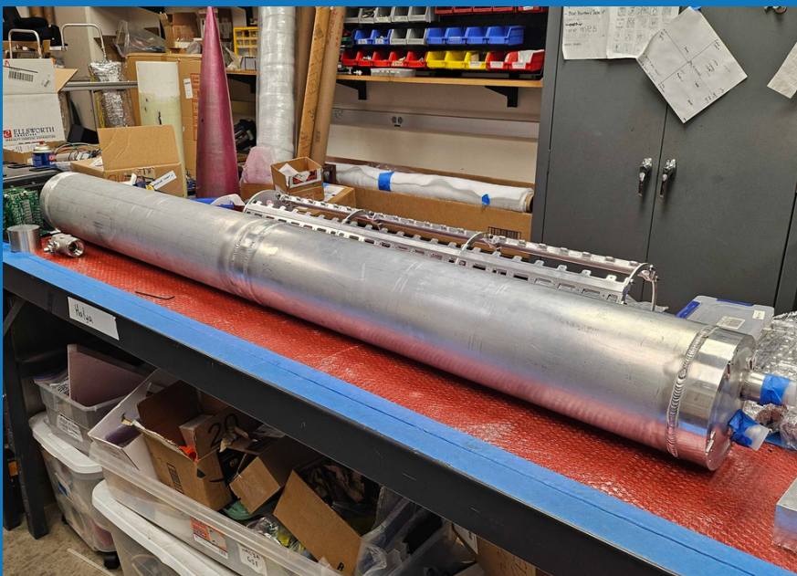
(Above) Halya's common bulkhead fuel and oxidizer tanks
